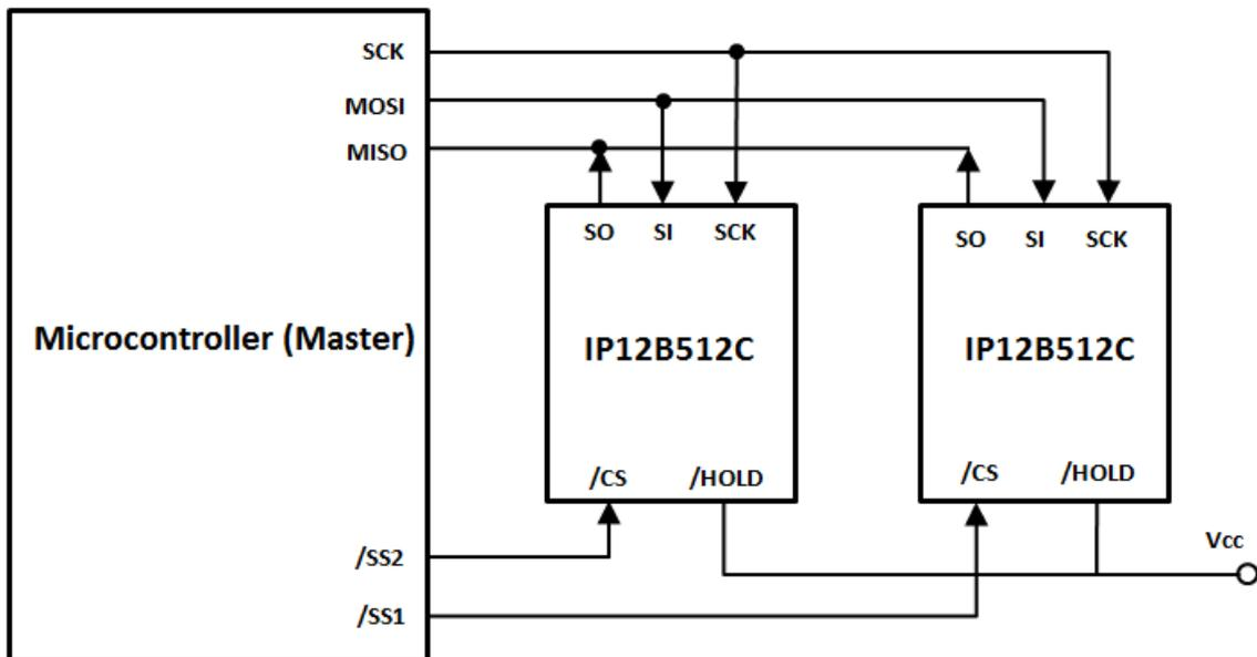
**Figure 3. System Configuration for two serial SRAM Devices (simplified schematic)**
